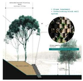
Due to the steep engineered slope, interlocking blocks were used to allow topsoil to be put in for planting purposes
